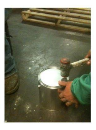
4.9 Secure the lid on the container using proper closing instructions.
