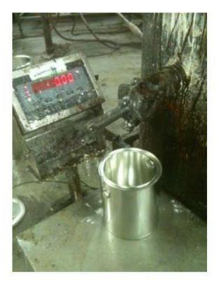
4.3 If the batch is to be short filled (filled to a specific weight with the use of a scale), zero the scale with the container on it. The QC Department will supply the information for the short fill.
