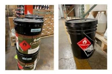
4.2.4 **Drum** - It is not common for Gemini to ship the product with a Class 3 and 8 combination in drums, so only the Class 3 Flammable product is shown below.
