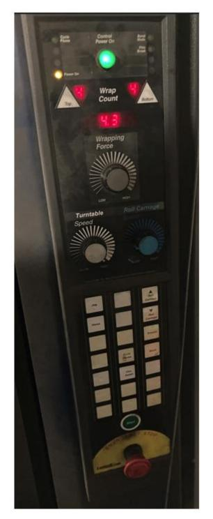
4.4.1 Wrapping Force – Used to tighten or loosen the strength of the wrap.
