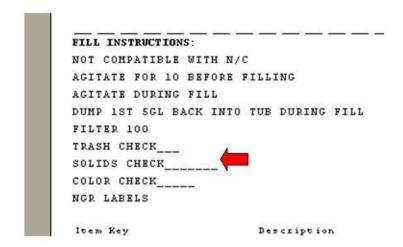
4.6 If the solids are not within the specified range, more product will have to be flushed through the machine and the process repeated.
