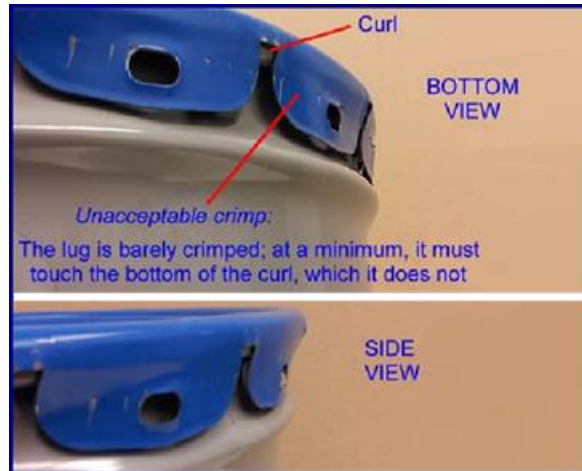
Figure 2: Unacceptable Crimp
